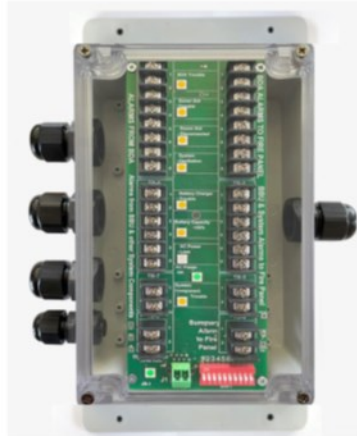
Figure 11. Optional Active Headend Alarm Splitter to Enable Easy Connection of DAS Components to both the Building's Fire Panel, Remote Modules and the DAS Alert Panel (includes LED Indicators and audible alarm Buzzer)
