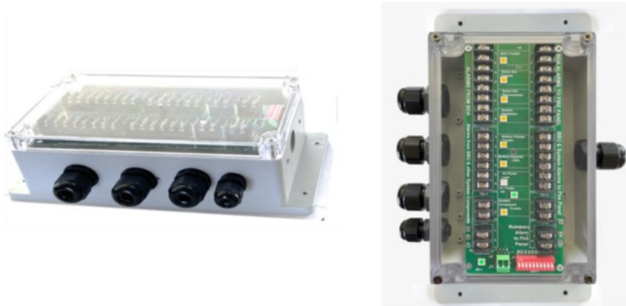
Figure 11. Optional Active Headend Alarm Splitter to Enable Easy Connection of DAS Components to both the Building's Fire Panel, Remote Modules and the DAS Alert Panel (includes LED Indicators and audible alarm Buzzer)
