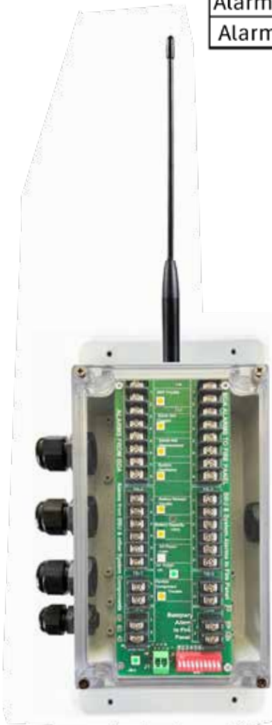
Headend Transmitter / Annunciator
